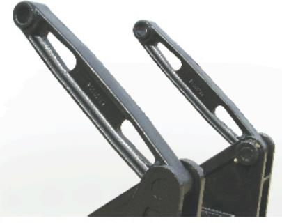
Shown is the heavy duty cast lift arms. These arms easily attach directly to the body using 4140 grade, 1 1/2" pivot pins which are bolted in place with grade 8 bolts.
