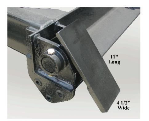
The hinges are cast from extra heave duty 4140 grade steel to ensure durability. Adding to the ease of installation and durability, these hinges are welded to the body's box-type long sills.
