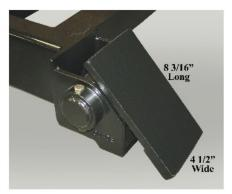
The 740U/750U's hinges are cast from extra heavy duty 4140 grade steel to ensure durability. Adding to the ease of installation and durability, these hinges are welded directly to the body's longitudinals.
