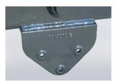
This hoist is easily installed to the trucks chassis using extra heavy duty 4140 grade cast mounting brackets. With 18 grade 8 bolts and minimal welding, installation is quick and easy.
