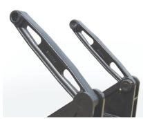
Shown is the heavy duty cast lift arms. These arms easily attach directly to the body using 4140 grade, 1 1/2" hinge pivot which are bolted in place with grade 8 bolts.
