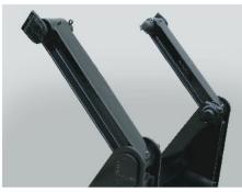
Shown is the U850D/U860D heavy duty cast lift arms. These arms easily attach directly to the body using 4140 grade, 1 1/2" pivot pins. The arms have easily accessible zerk grease fittings.
